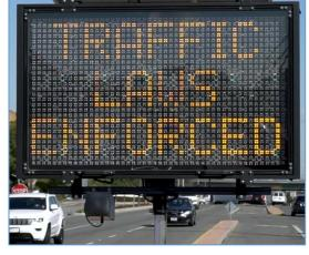
Additionally, a message board was deployed with an onboard computer which collects data on the number of vehicles traveling on the road and the speed at which the vehicles are traveling. What was observed by the motor officers, and supported by the data collected, was during the drop off and pick up times traffic in the area was too congested to allow for excessive speeds and the drivers appeared to be driving in a safe manner.
