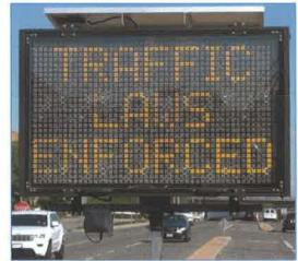
Additionally, a message board was deployed with an onboard computer which collects data on the number of vehicles traveling on the road and the speed at which the vehicles are traveling. What was observed by the motor officers, and supported by the data collected, was during the drop off and pick up times traffic in the area was too congested to allow for excessive speeds and the drivers appeared to be driving in a safe manner.
