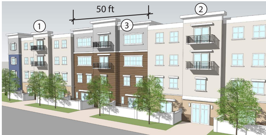
Roof Line Variation
