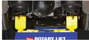
Adjustment range and rotated adapters with an off-set transaxle.
