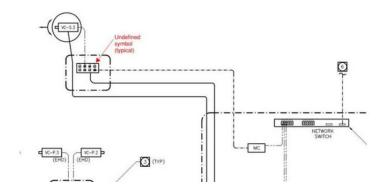
**A6b:** The referenced device in the drawing attached to the Bidder's RFI (partial, marked up portion of plan shown above) is a hardened outdoor rated switch. It is specified in Section 282300, Article 2.2, Paragraph B.
