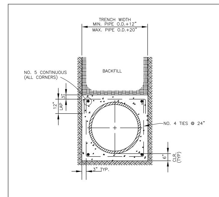
CONCRETE ENCASEMENT DETAIL
