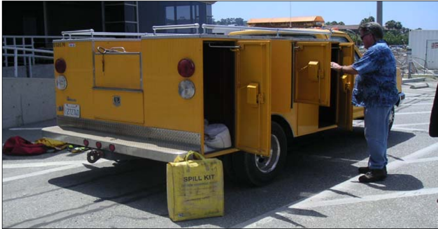
Airport Operations Vehicle: The airport operations vehicle is equipped with fire extinguishers, tool-boxes, and other materials needed to respond to minor accidents.
